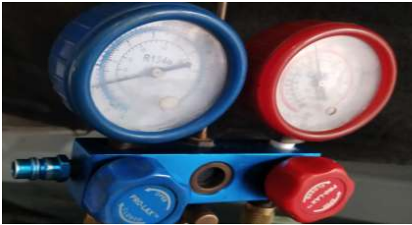
Charging & Discharging of refrigerant Machine in car AC.
